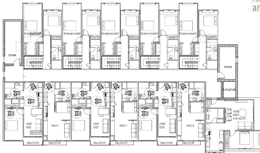
1 SECOND FLOOR Scale: 1:128 3 BACH. FLOR. - 434 SQ.FT. 3 - ONE BEDROOM - 673 SQ.FT. 1 - ONE BEDROOM - 674 SQ.FT. 5 - 2 STOREY TOWNHOUSE - 1246 SQ.FT.
